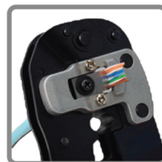
Special tool to crimp and cut the extra cores in one press
